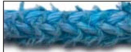
FIG. 3 Severely abraded rope
