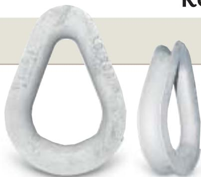
The cast steel extra heavy duty hawser thimble is designed for use with wire rope or high performance synthetic fiber ropes such as Amsteel Blue, Force 8, & DPX 75. The galvanized thimble provides smooth even grooves, maximum strengths at critical areas, and proper bending radius for the rope. When used with synthetic ropes, thimble eye should be lashed at approximately 2, 4, 8, & 10 o'clock on the thimble circumference to secure the thimble to the rope when not in service.
