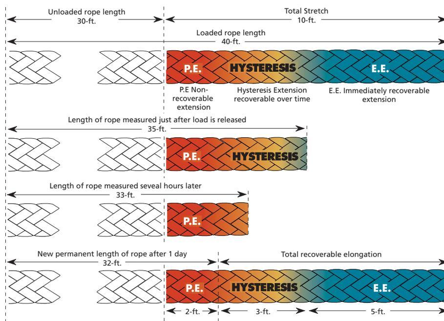
**PUBLISHED ELASTIC ELONGATION DATA: ALL REPORTED PERCENTAGES ARE AVERAGES BASED ON TESTS OF NEW ROPE STABILIZED FROM 200D<sup>2</sup>. TESTED ROPES ARE STABILIZED BY BEING CYCLED 50 TIMES AT EACH STATED PERCENTAGE OF ITS AVERAGE BREAK STRENGTH.**
