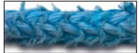
FIG. 3 Severely abraded rope
