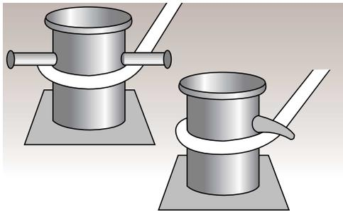
Many tugboats using eight and nine-inch circumference headlines in ship-handling work have fair size bitts (eighteen-inch diameter, etc.) which is an adequate bending radius. However, ironically, many of these bow and shoulder bitts are equipped with "horns" of a relatively small diameter (five or six-inches) and it is these horns under or over which the lines pass and bend first in many cases. This results in shortened rope life and excessive rope replacement costs.
