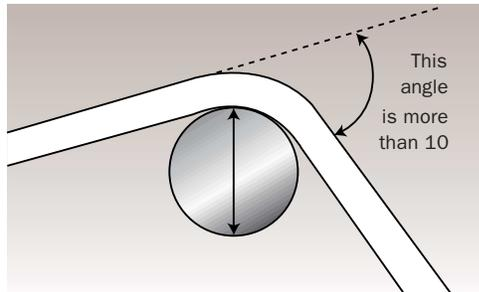
Where a rope bends more than ten degrees around bitts or chocks or is bending across any surface, the diameter of that surface should not be less than three times the diameter of the rope. Stated another way, the diameter of the surface should be at least three times the rope diameter. A four-to-one ratio (or larger) would be better yet because the durability of the rope increases substantially as the diameter of the surface over which it is worked increases.
